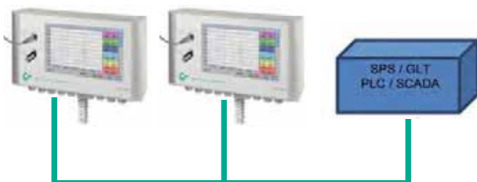
RS 485 network (Modbus RTU) or Ethernet (Modbus/TCP)
