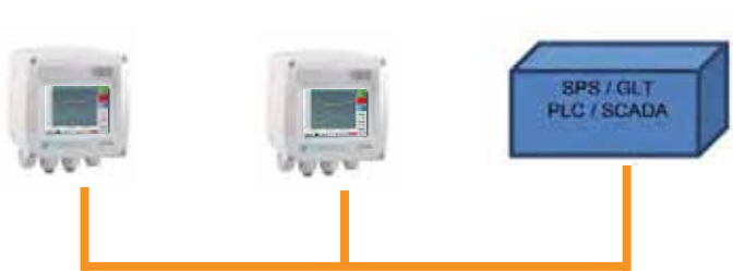
RS 485 network (Modbus RTU) or Ethernet (Modbus/TCP)
